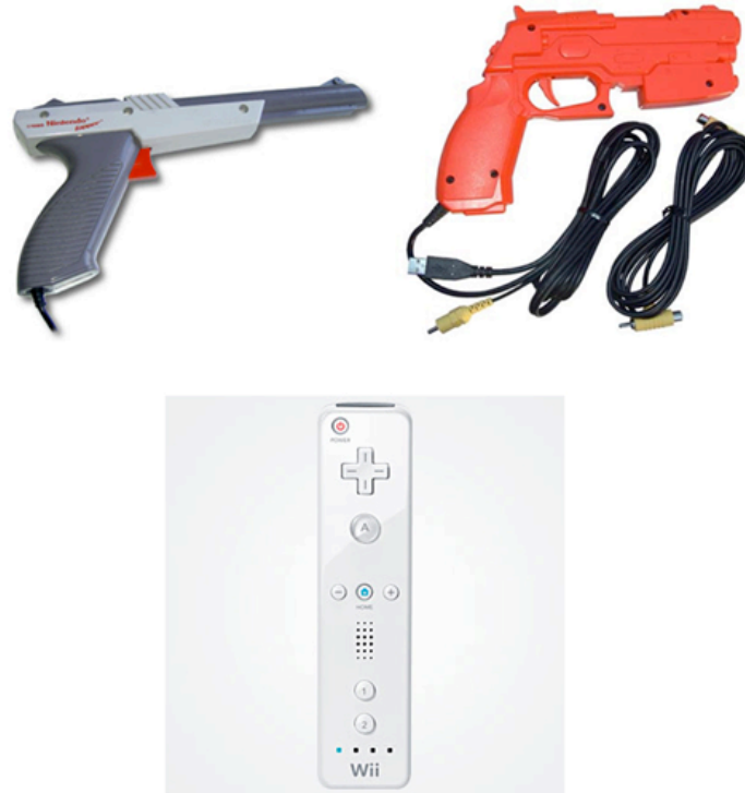
Figure 2: Examples of light-based controller systems used for 3D video games. Top-left: Nintendo Zapper; Top-right: Namco GunCon; Bottom: Nintendo Wii Remote
