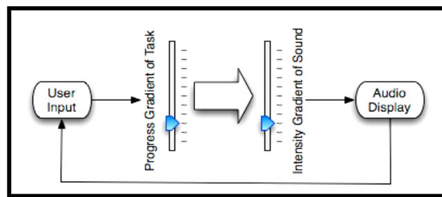
Figure 3. Illustration of the intensity-based auditory feedback model
