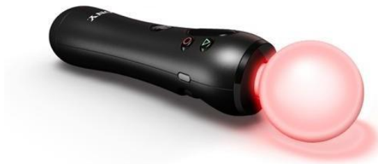
Figure 3 : The Move wand, showing the illuminating sphere used to track it. These vary in color, and allow the wand to be used as a pointer.
